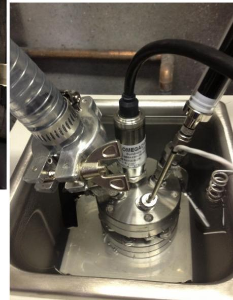
Reid vapor pressure and  $T_{V/L=20}$  testing chamber
