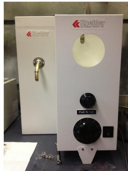
ASTM D86 Distillation Apparatus
