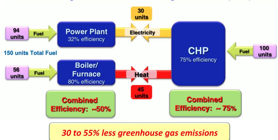
CHP delivers major boost in energy efficiency while simultaneously significantly reducing CO<sub>2</sub> emissions
