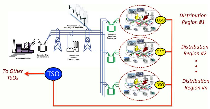
Proposed DDS architecture is conveniently scalable over a wide range of grid sizes and configurations
